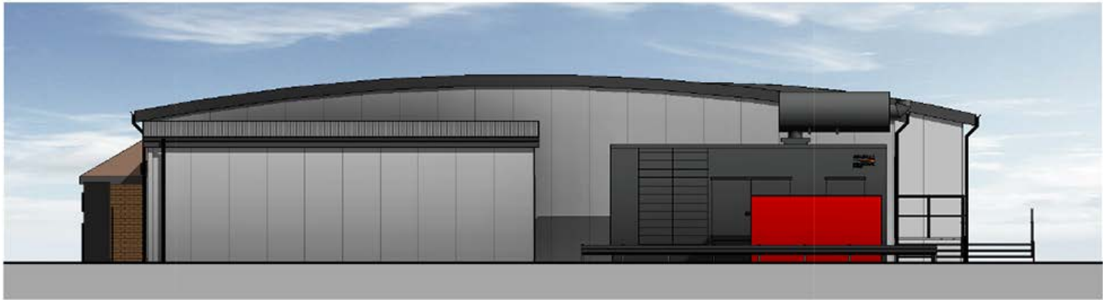
External ModuSec panels onto internal steel frames with standing seam steel tray roofs
