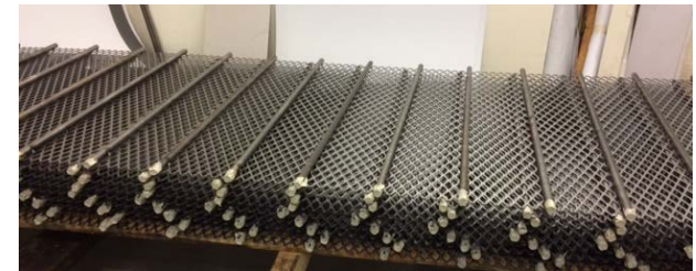
Mesh foamed into in panels
