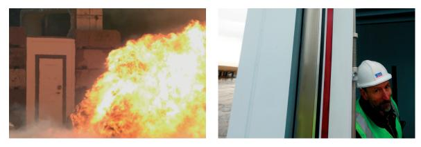
Same enclosure rotated and re-tested C15: 15m standoff. Peak Pressure: 290 KPa. Peak Impulse: 1023 KPa
